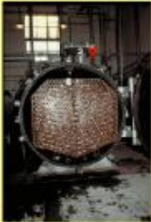
In a batch retort, carts loaded with canned food are pushed into the retort. The retort lid is closed and steam is turned on. After a desired heating period, the steam is turned off, cooling water is introduced to cool the cans. The retort lid is opened and carts are pulled out of the retort.
